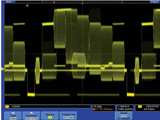
Figure 6. An NTSC composite video signal is an example of a complex wave.
