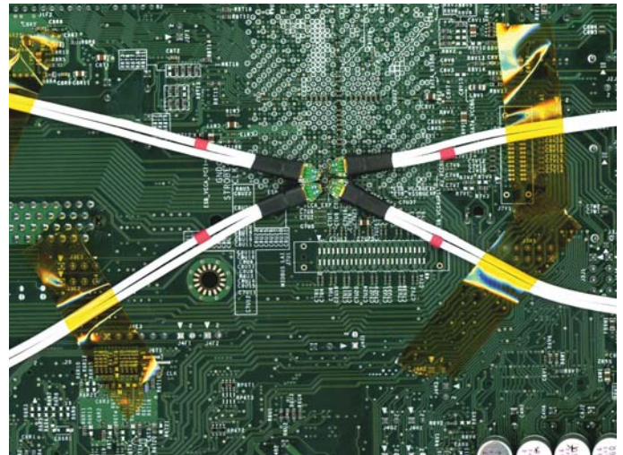
Figure 38. Dense devices and systems require small form factor probes.
